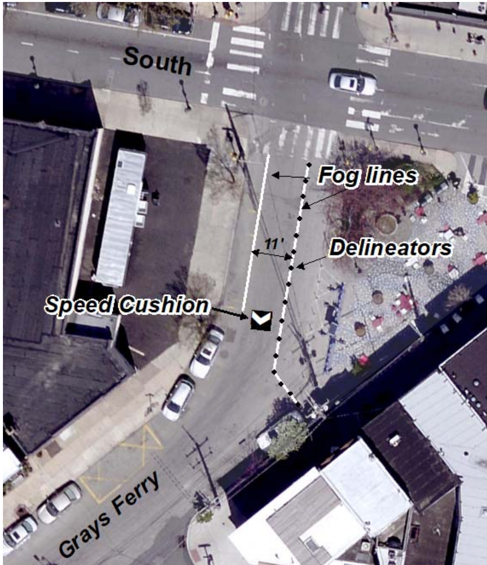
Speed cushion, fog lines, vertical delineators
